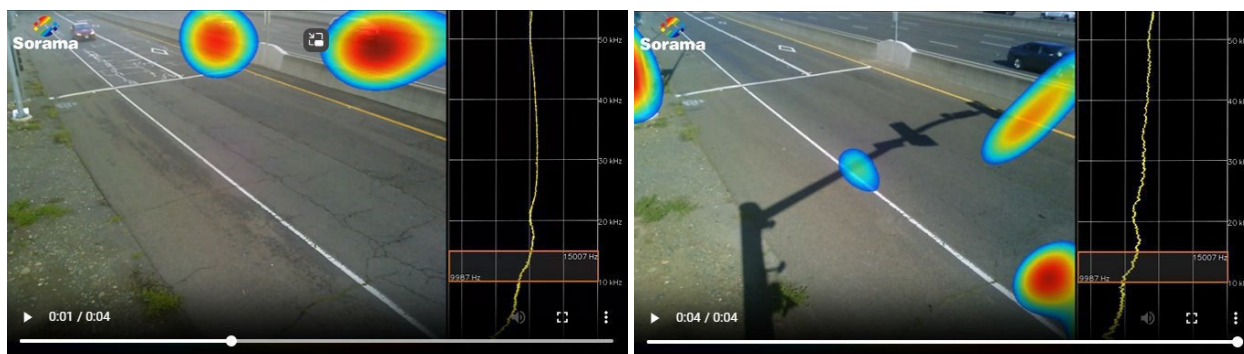
Figure 5. Still Images from Video Recordings Displaying Sound Intensity Arrays Tracking Multiple Vehicles in the Same Event (left) and Sound Intensity Arrays Not Tracking a Vehicle (right).
