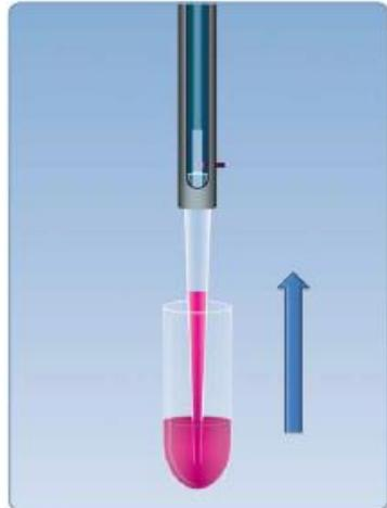
Figure 1: Aspiration from a sample tube
