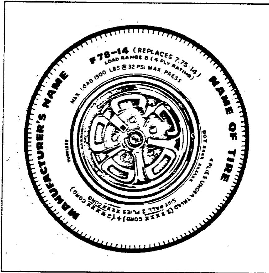
Fig. 1-15. New Passenger Car Tire Marking
