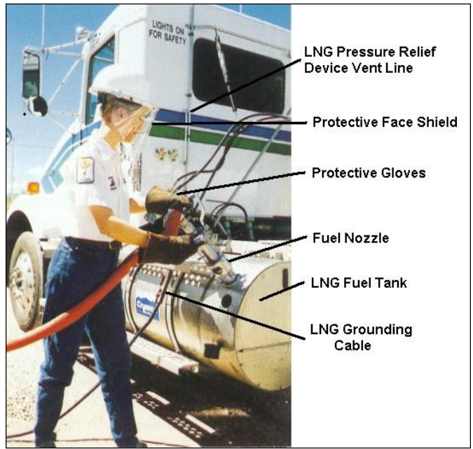
Figure 11-41e. Safety Items Associated with LNG Fueling
