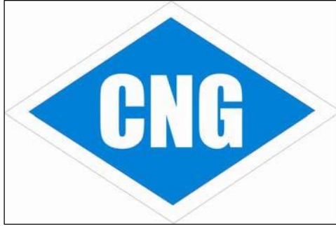
Figure 11-37. CNG Label Required by NFPA 52
