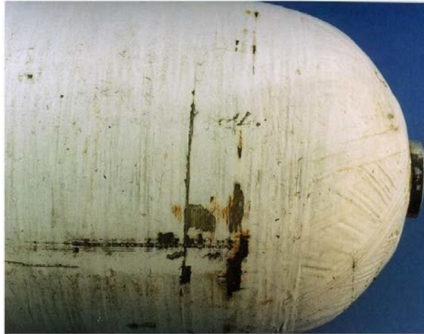
Figure 11-15a. Type 3 Container with Level 1 Abrasion Damage from Mounting Bracket
