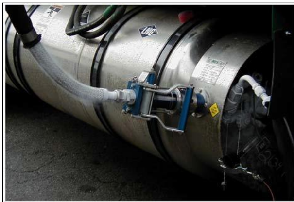
Figure 11-42l. Fuel Fill Fitting
