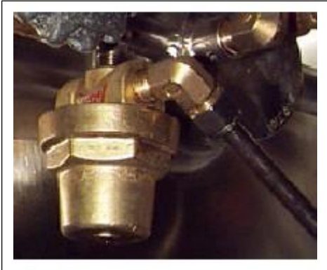
Figure 11-42g. Pressure Control Regulator
