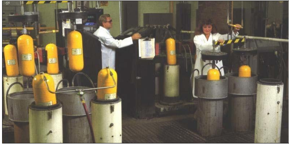
Figure 11-6. Typical Manufacturer's Container Hydrostatic Test
