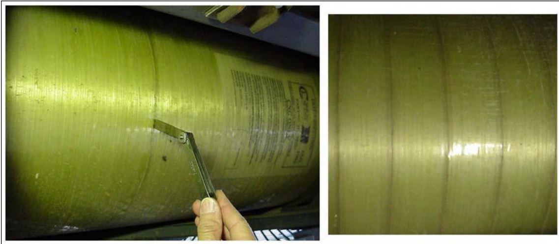
Figure 11-16a. Type 2 Container Composite Cracking or Separations are Not Considered as Damage
