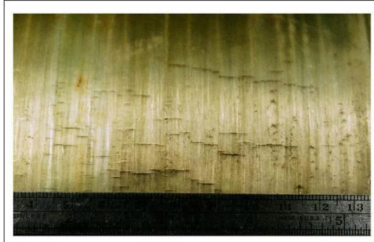
Figure 11-17. Level 3 Chemical Damage to Container (Stress Corrosion Cracking)
