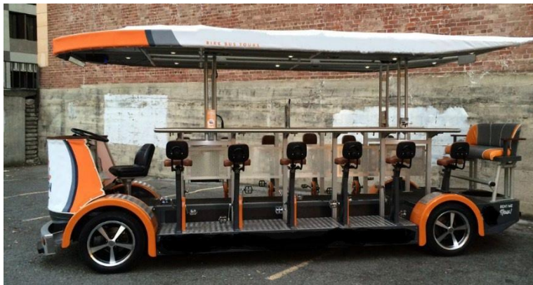
Figure 4-4. Example of a party bike pedicab as defined in Section 467.5(c) CVC.
