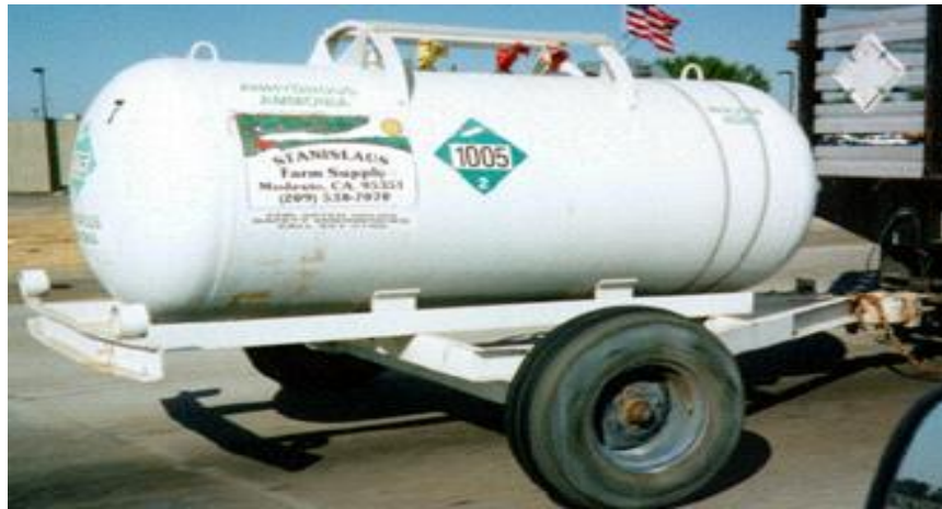
Figure 9-13 Anhydrous Ammonia Trailer
