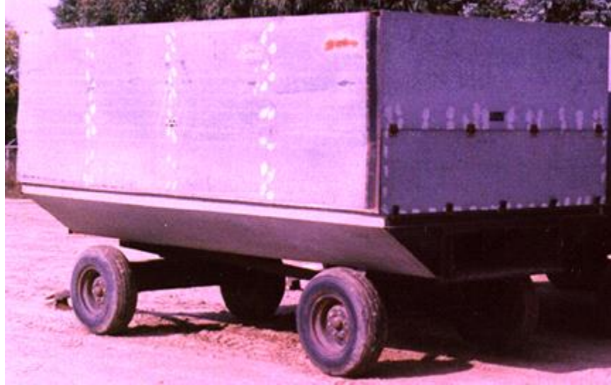
Figure 9-42 Plenum Chamber Trailer
