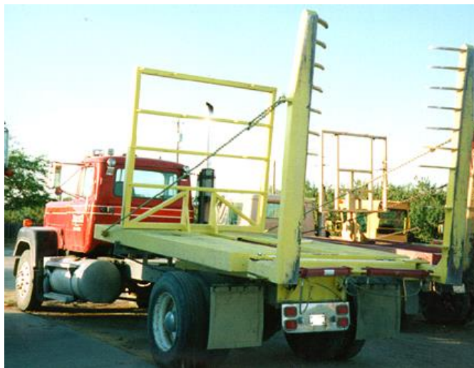
Figure 9-24 Truck-Mounted Stack Retriever
